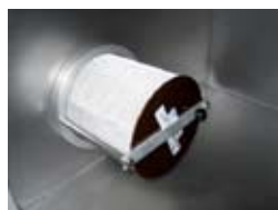
H13 HEPA filter air inlet and outlet
